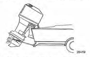
IMPORTANT: Do not rely on the power trim/tilt system or tilt support lever to maintain proper ground clearance for trailering. The outboard tilt support lever is not intended to support the outboard for trailering.
