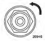
3. Set the spark plug gap to specifications.
