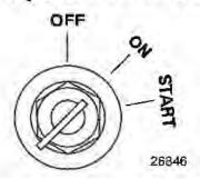
Within the first 10 seconds after the key switch has been turned on, move the remote control handle from neutral into forward gear 3 to 5 times. This will automatically start the priming process.
