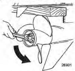
Pull the propeller straight off the shaft. If the propeller is seized to the shaft and cannot be removed, have the propeller removed by an authorized dealer.
