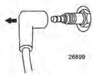
Remove the spark plugs to inspect. Replace spark plug if electrode is worn or the insulator is rough, cracked, broken, blistered, or fouled.
