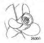
Place a block of wood between the gearcase and propeller and remove the propeller nut.
