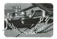
Criss-Cross the trailer safety chains underneath the trailer tongue.
